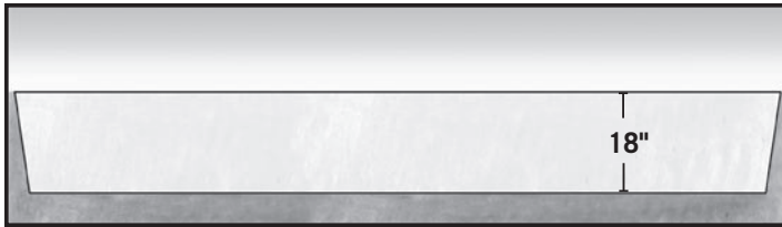
Fig. 3 First, dig entire basin to 18" depth.
