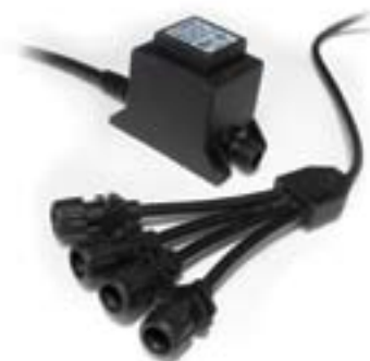
Model: SOL20X4 Description: Transformer and 4-way Splitter For Use With: Warm White AWG and SOL Lighting Voltage: 12 volt AC / 2-wire Watts: 20 Includes: Transformer and 4-way splitter w/ quick-connect plugs
