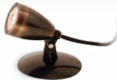
Model: SOLW6 Description: Warm White Spotlight Input Voltage: 12 volt AC Watts: 6 Includes: LED Spotlight, 20' power cord w/ quick-connect plug, stand and ground stake
