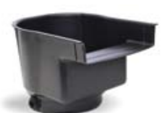
Model: BF1500 Waterfall Width: 20 1/2" spillway Dimensions: 24"W x 30"D x 20"H Pump Flow Range: 2,500 - 4,000 gph Bulkhead: 1 1/2" Match to Skimmer: PS4500 Includes: Retail packaging *no top grate
