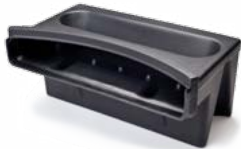
Model: SP1600 Waterfall Width: 16" Dimensions: 16½"W x 9½"D x 7¼"H Max Pump Flow: 3,000 gph Bulkhead: 1½" FIPT Application: Pond-free
